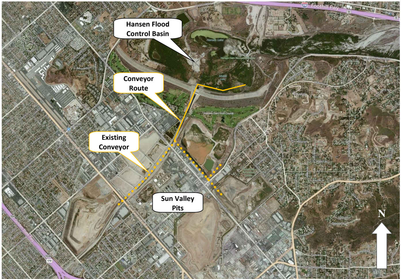
Figure 8-12 Potential conveyor alignment between Hansen Flood Control Basin and pits in Sun Valley
