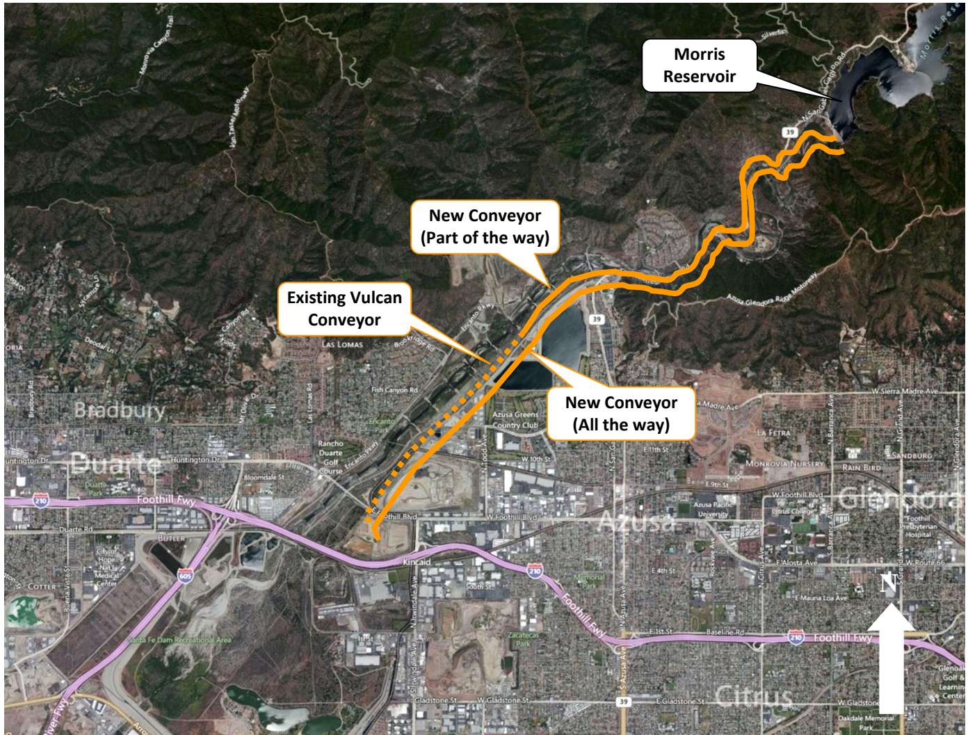
Figure 7-45 Morris Conveyor Belt Alignment
