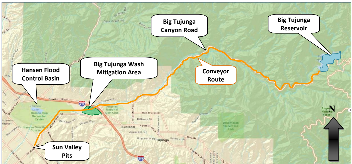
Figure 8-11 Potential conveyor alignment between Big Tujunga Reservoir and pits in Sun Valley
