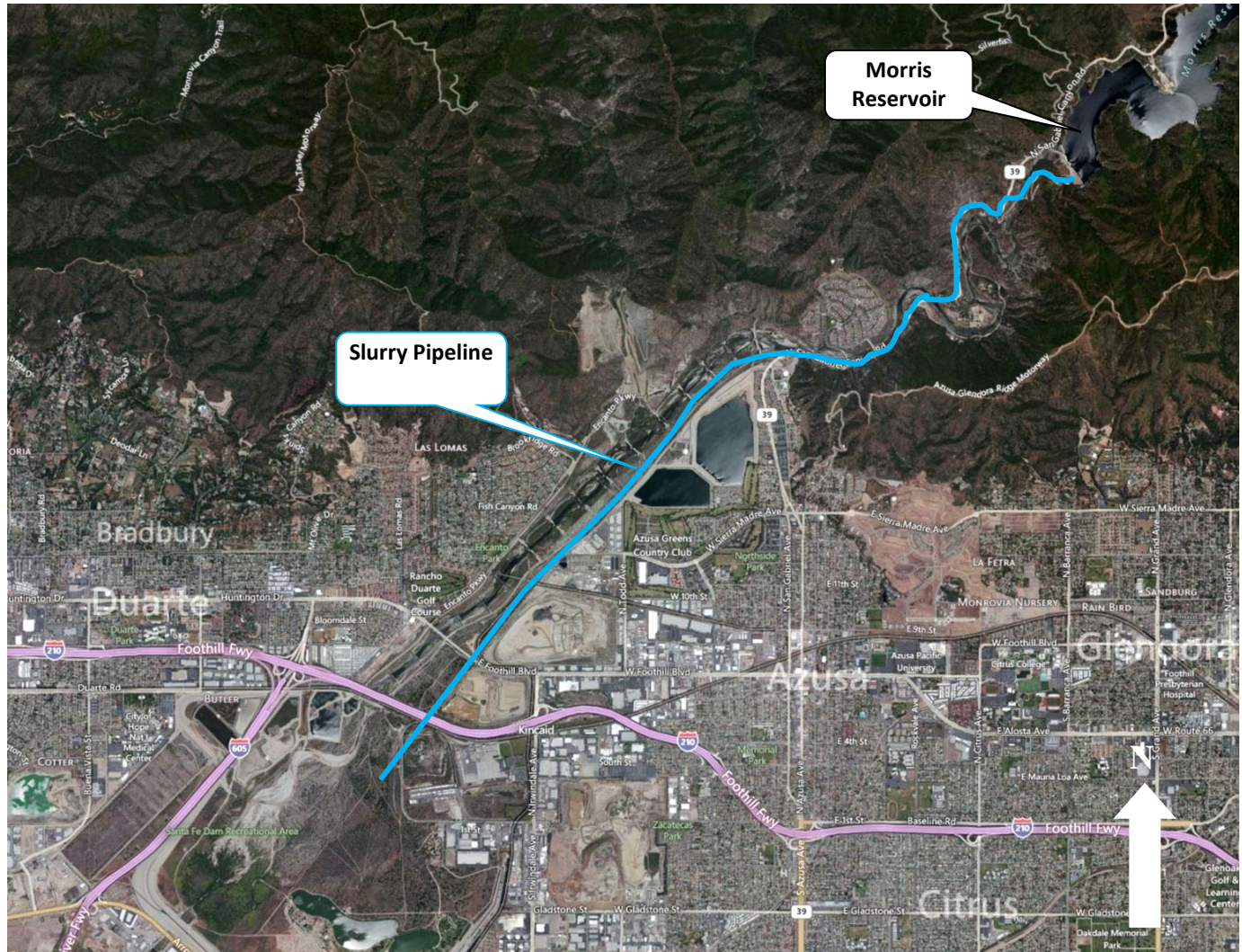
Figure 7-46 Morris Slurry Pipeline Alignment
